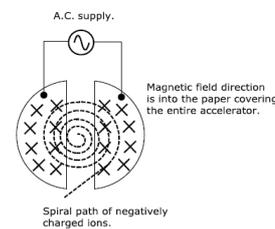
Figure 2 - Cyclotron
