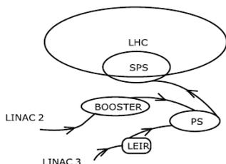
Figure 3 – Schematic diagram of CERN accelerators
